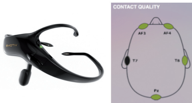
Picture 3. a. Brain signals recording emotiv tool, b. Positions of electrodes according to brain structure
